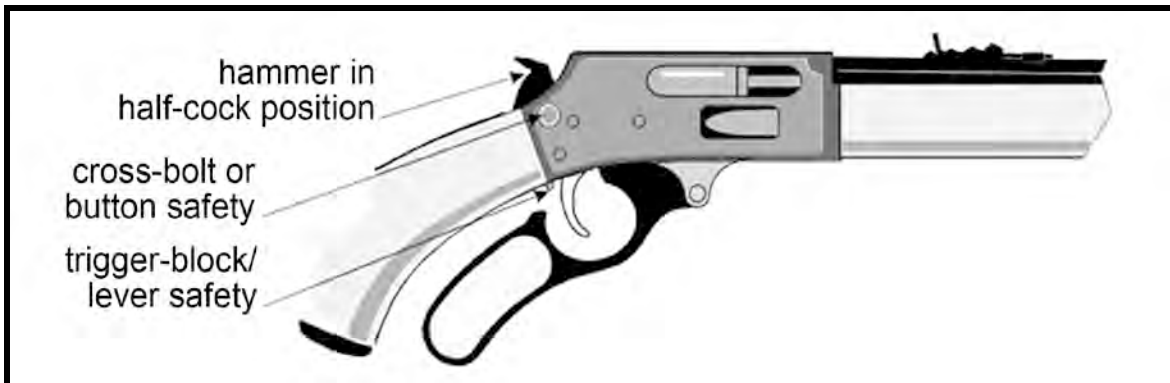
Figure 44. Trigger block/lever safety
